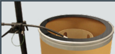
Top view of turn table showing wire guide
