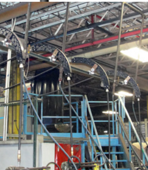
Large 90° Guide Modules® installed in a submerged arc welding application
